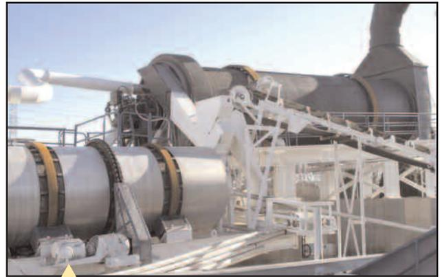
*A secondary mixing drum that is used to blend the RAP and virgin components is shown on the left. The primary dryer is on the right.*
