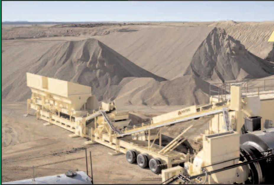
*RAP can be introduced into the mix via an integrated, in-line feeding system.*
