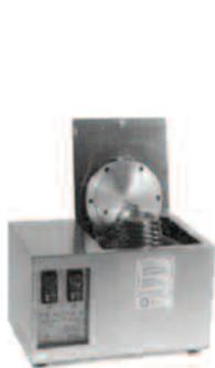
Prentex PR9300 Pressure Aging Vessel
