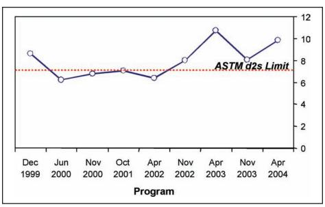
FIGURE 3: REPRODUCIBILITY LIMITS (d2s) FOR PENETRATION AT 77°F (25°C)
