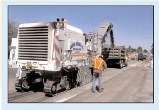
The *Wirtgen W 2000* from Wirtgen America is a high-performance, large-volume, compact milling machine with broad cutting width for removing deteriorated asphalt pavement or complete roadway structures down to 13 inches in a single pass. The W 2000 boasts a 565 hp engine and features front loading of RAP for ease of operations. It has a base cutting width of 79 or 87 inches, can operate at speeds up to 180 fpm, and has an operating weight of approximately 64,000 pounds.
