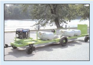
The patented *Ray-Tech Joint Heating System* effectively eliminates longitudinal cold joint failure by providing 98-100 percent density at the joint. The infrared heating system is capable of indepth heating of longitudinal joints without burning or damaging the asphalt. This complete system is a proven, effective method of eliminating joint failure.
