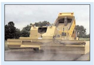
Etnyre Chip Spreaders are designed to spread aggregate in the chip seal process. The spreaders feature controlled application rates and have individual one foot wide power gates across the entire spreader width. Engine options range from 200 to 240 hp and the chip spreaders are available in front wheel or four wheel drive models.
