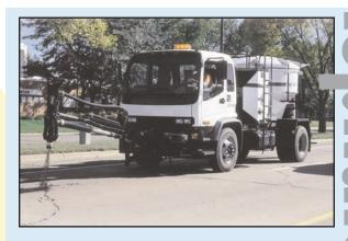
The *Rosco RA-300 Spray Injection Patcher,* with its one-person, from-the-cab operation makes safely and effectively repairing potholes a year-round activity. The RA-300 features its in-cab controls, full-function spray nozzle with joystick control and front-mounted patching boom and rear-mounted arrowboard for maximum simplicity, effectiveness and safety. Its hydraulic "Patch-on-the-Go" feature allows for patching on the move with no auxiliary power.
