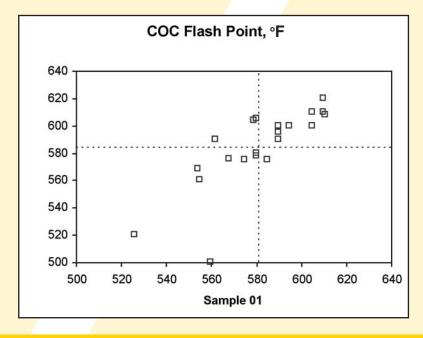
This scatter diagram illustrates the variability of test results obtained for the flash point of two roofing asphalt samples.
