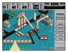
Graphical user interface (GUI) for control of an asphalt plant
